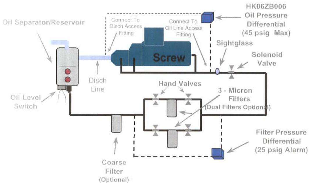
While running the oil pressure differential switch will see high side pressure on both connections
