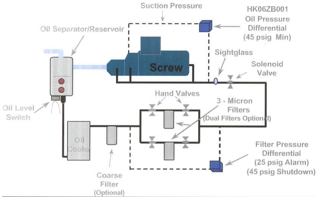
As used today, the oil pressure differential switch sees oil pressure (high side) on the high connection and suction pressure on the low connection. The differential can be as high as 320 psid.
