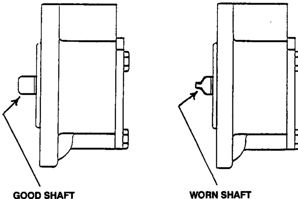
**NOTE:** It may appear that the crankshaft is also worn. This is NOT the case. The conical shape to which the oil pump shaft wears is due to the center drilling in the end of the crankshaft that is necessary to machine the crankshaft. The crankshaft is much harder than the pump shaft and will not wear.
