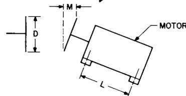
Retighten holddown bolts and recheck. Readjust the motor position, if necessary, until the total indicator reading is within the allowable variation shown in Table 2.
