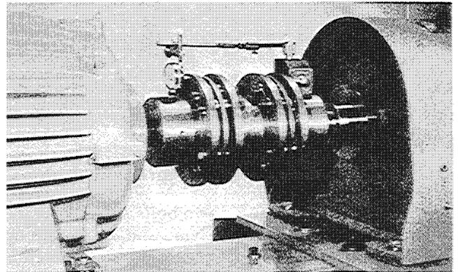
**Fig. 5 — Set-Up for Checking Angular Alignment**
