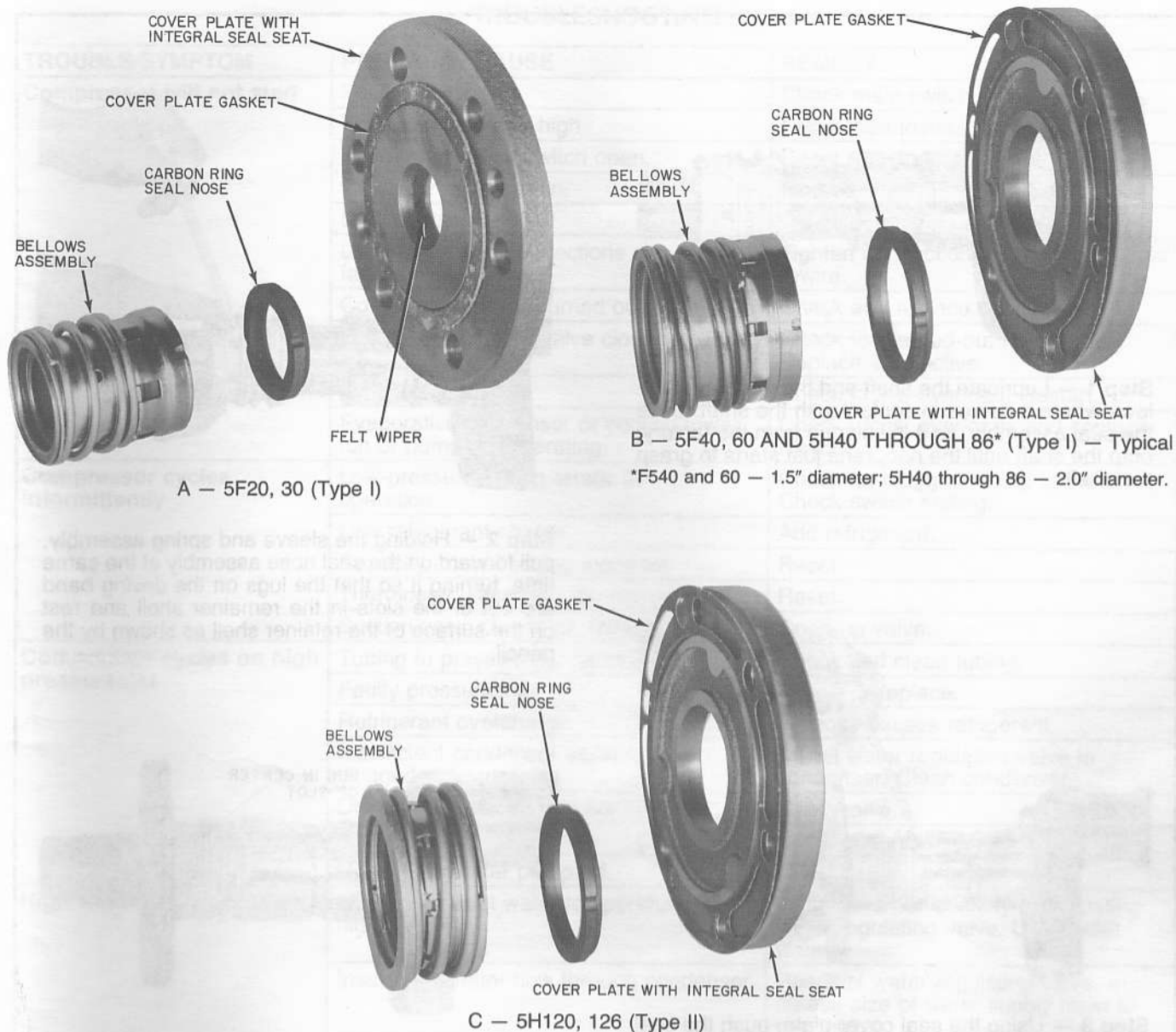
Fig. 50 — Service Replacement Seals
