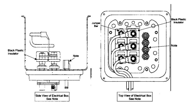
NOTE: 06T terminal arrangement shown. The 06E and 06CC (50-99 cfm) terminal box may or may not have three electrical posts in place of the 4 thermistor pins shown above.
