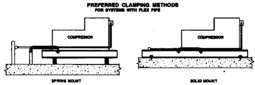
NOTE: ONLY DETAILS WHERE CLAMPS SHOULD BE PLACED IN RELATION TO PLEX PIPE, NOT ALL PIPING.
