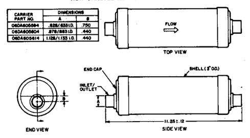
Mufflers are typically not needed in system designs. Reciprocating compressors emit gas pulsations and these pulsations sometimes react with specific system designs and cause vibration. In these systems where pulsation driven vibration has proven to be a problem, a properly sized muffler should be used.
