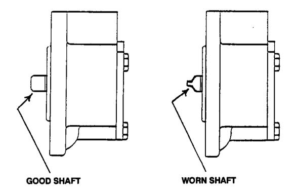
**NOTE:** It may appear that the crankshaft is also worn. This is NOT the case. The conical shape to which the oil pump shaft wears is due to the center drilling in the end of the crankshaft that is necessary to machine the crankshaft. The crankshaft is much harder than the pump shaft and will not wear.
