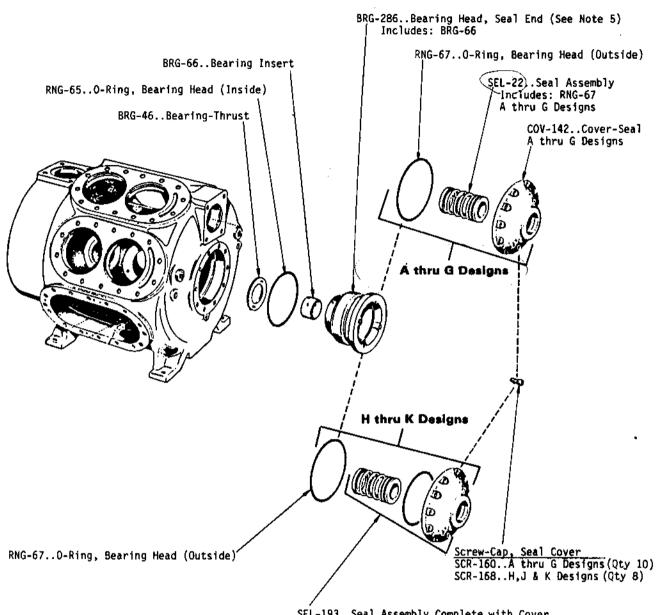
SEL-193..Seal Assembly Complete with Cover Includes: GKT-170..Gasket-Cover H,J & K Designs (See Note 5a)
